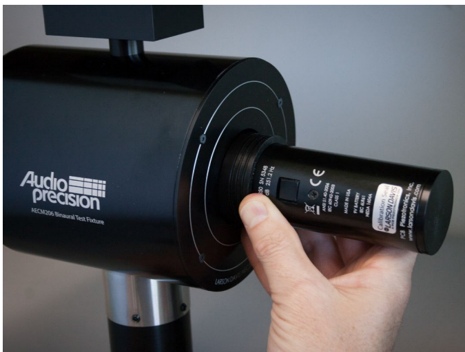
Figure 17. A CAL250 sound level calibrator is used to calibrate the ear simulator microphones.
